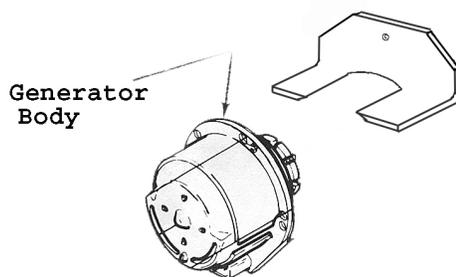
2" x 3/16 Angle Aluminum Saddle cut to accept Generator body. Angle aluminum then attached to Generator body using 3" Hose clamps. Angle mount then bolted to aircraft
